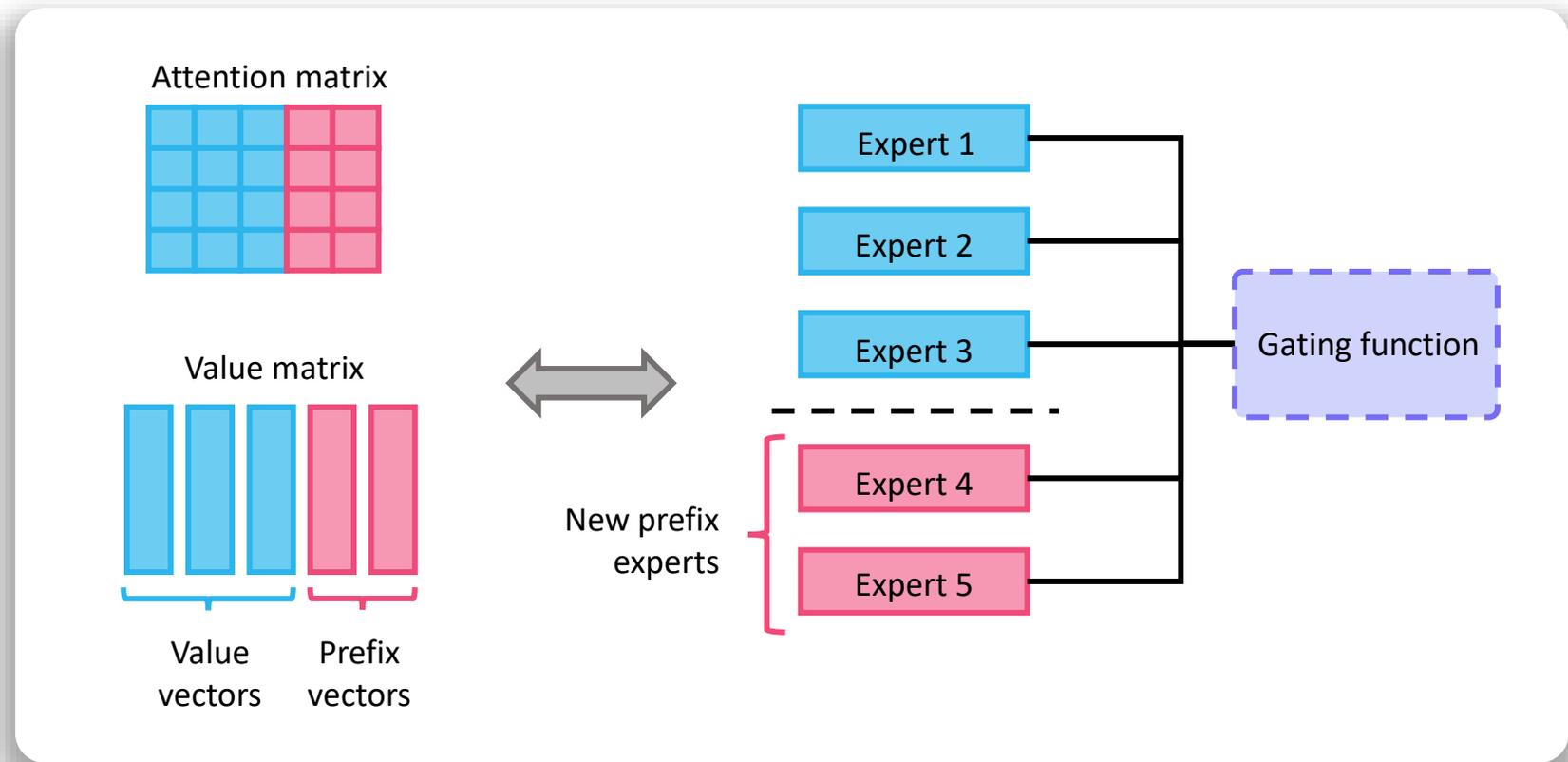
$$\tilde{\mathbf{h}}_l = \text{Attention} \left( \mathbf{X}^Q W_l^Q, \begin{bmatrix} \mathbf{p}^K \\ \mathbf{X}^K \end{bmatrix} W_l^K, \begin{bmatrix} \mathbf{p}^V \\ \mathbf{X}^V \end{bmatrix} W_l^V \right) = [\tilde{\mathbf{h}}_{l,1}, \dots, \tilde{\mathbf{h}}_{l,N}]^\top \in \mathbb{R}^{N \times d_v},$$
