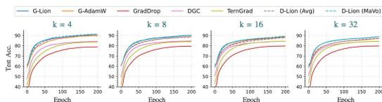
Performance of Distributed Lion v.s. baseline distributed optimizers on CIFAR-10 with 4, 8, 16, and 32 workers, each worker at each step runs on a local batch with size 32.
