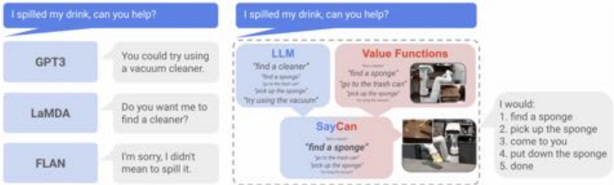
Figure 1: LLMs have not interacted with their environment and observed the outcome of their responses, and thus are not grounded in the world. SayCan grounds LLMs via value functions of pretrained skills, allowing them to execute real-world, abstract, long-horizon commands on robots.
