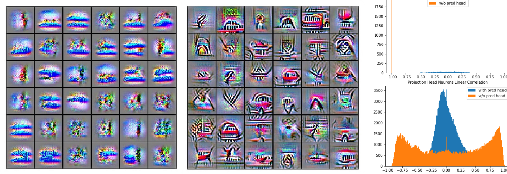
Visualization of intermediate features in Wide-ResNet. Left: dimensional collapsed features, all features are alike; Middle: well-generalizing features, which are diverse and semantic; Right: neuron correlations of projection head features or encoder features.
