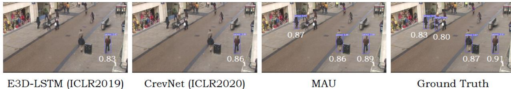
Figure 5: Object detection experiments on the predictions (4 frames → 1 frame) from different methods using Yolov5s pre-trained model [41]. Confidence threshold is set to 0.8.
