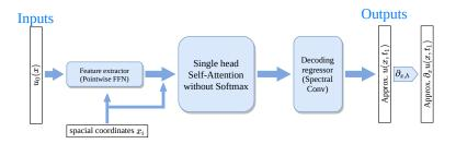
A simple attention-based "encoder-decoder" mimicking the ones in NLP.
